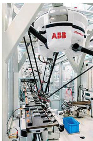
Figura 2.12 ABB IRB 360 FlexPicker Delta
