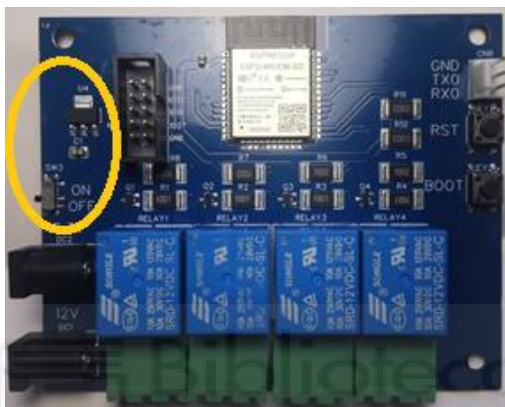
Figura 7.9 Interruptor y convertor DC-DC
