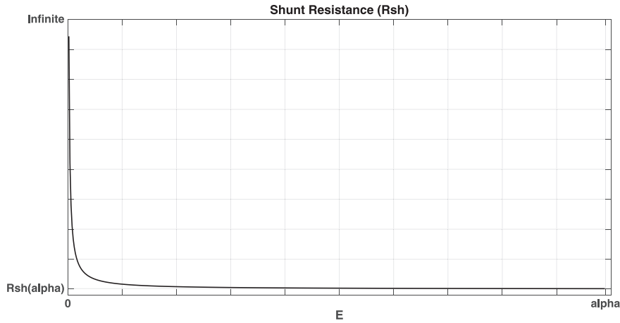
Fig. 5. The shunt resistance R_{sh} in \Omega as a function of E in [\Omega^{-1}] .
